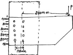
Design a battened column with two channel back to back of length 10 m to carry an axial factored load of 1400 KN. The column may be assumed to restrained in position but not in the direction at both ends. (12.5)
