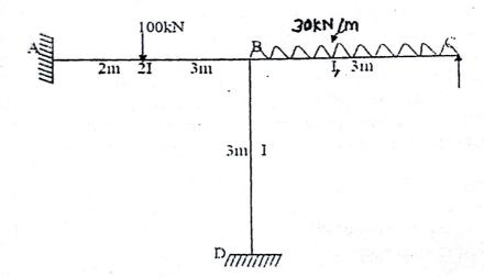
Q4. For a cantilever beam of uniform cross section shown in figure, develop the flexibility and stiffness matrices with reference to the coordinates. Verify that the two matrices are the reciprocal of each other.
